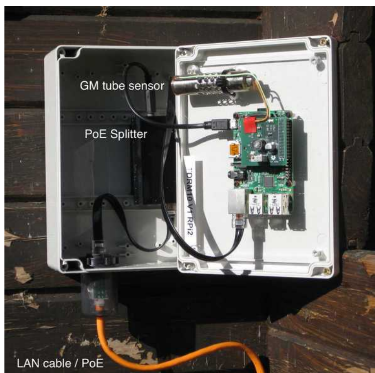
Fig. 3: Computer board, on top PIN diode sensor (left), sensor box with GM counter tube (right)
